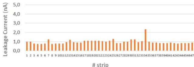
Fig. 3. The surface current of the detector D3 is acquired after the bonding process.
